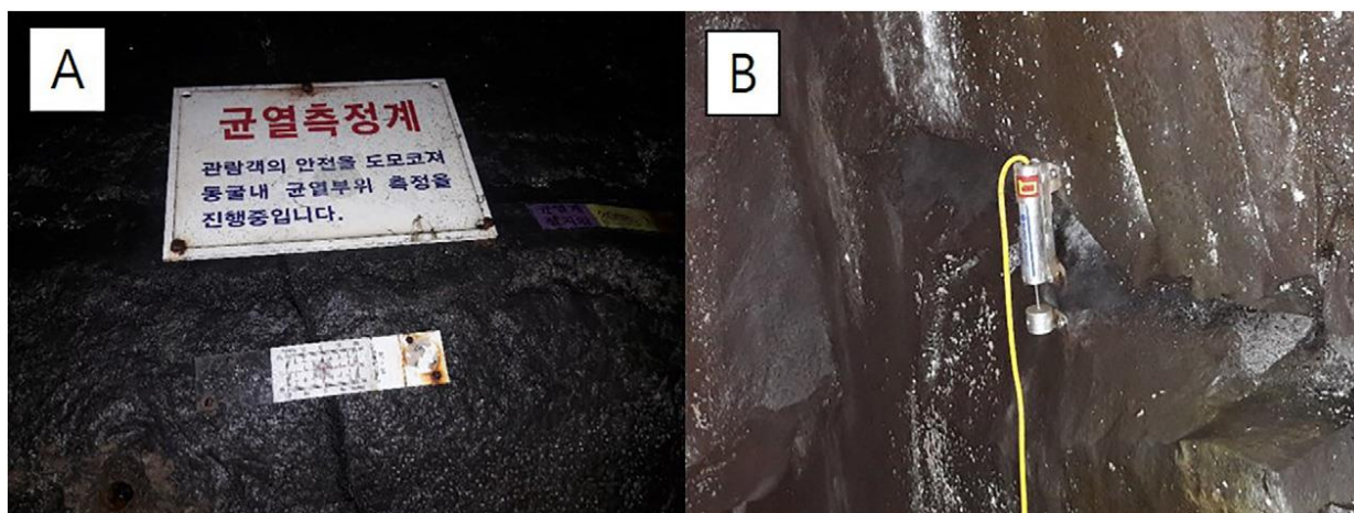
Figure 51 – Crack monitoring using glass plate (A) and monitoring gauge (B) in Manjanggul Cave (lava tube), Jeju Island, Korea (Woo and Worboys, 2019).
